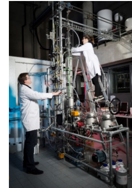
Pilot-scale rectification column at HEIA-FR
